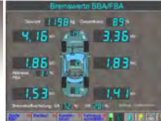
Distinct display of all measurement values with PC-Software MPP-Basic
