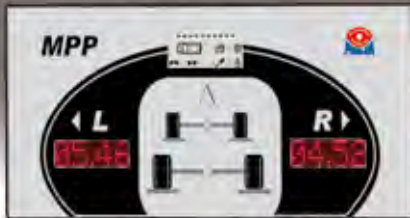
Display of the measurement values with bright LED digital display
